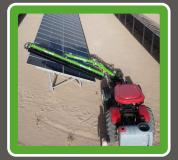
These brushes enable efficient cleaning of solar systems, regardless of the orientation or tilt angle of the solar modules:
